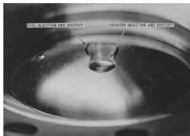
**Figure 17. Face Shutoff Pintle Injector in Closed Position**
