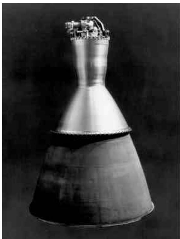
**Figure 14. TRW's TR201, Derived from LEMDE, was Used as the Delta Upper Stage with a 100% Flight Success Rate**
