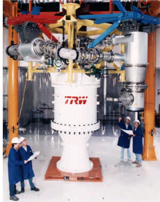
**Figure 26. The 650,000 lbf LOX/LH2 Low Cost Pintle Engine (LCPE) . . . the Largest Pintle Engine Built to Date**
