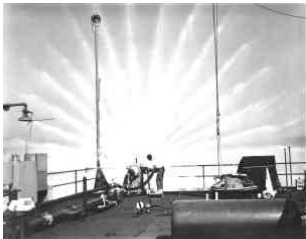
**Figure 15. Water Flow Test of Pintle Injector for Air Force 250,000 lbf Engine**
