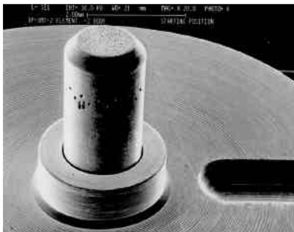
**Figure 21. Pintle Injector on Brilliant Pebbles 5 lbf Engine**
