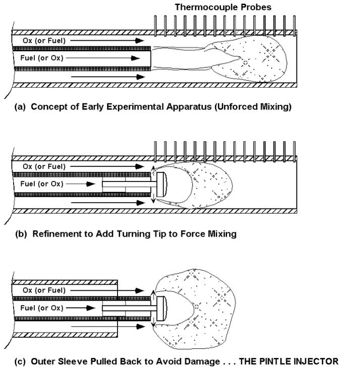
**Figure 5. Evolution of JPL Laboratory Apparatus for Studying Reaction Rates and Combustion Phenomena of Hypergolic Propellants**
