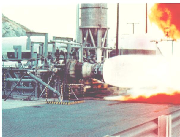
**Figure 16. Hot Fire Test of Pressure-Fed 250,000 lbf Ablative Engine**
