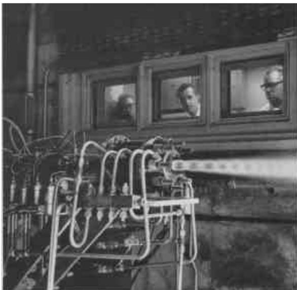
**Figure 8. Test Firing of Earliest TRW Pintle Injector Engine, a Water-Cooled MIRA 500**
