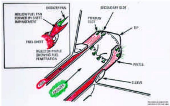
**Figure 2. Pintle Injector Concept (Slotted Injection, Fixed Thrust Design)**
