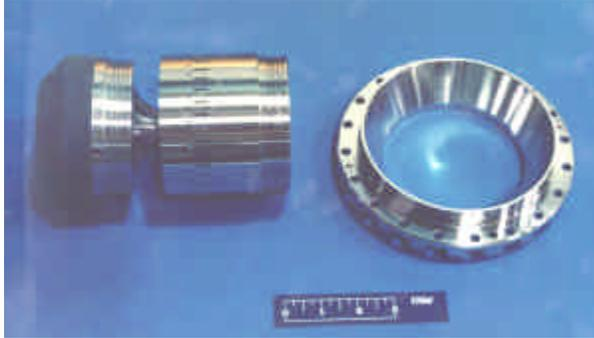
**Figure 23. Pintle Tip, Oxidizer Orifice Ring and Fuel Gap Ring from 16K LOX/LH2 Engine**
