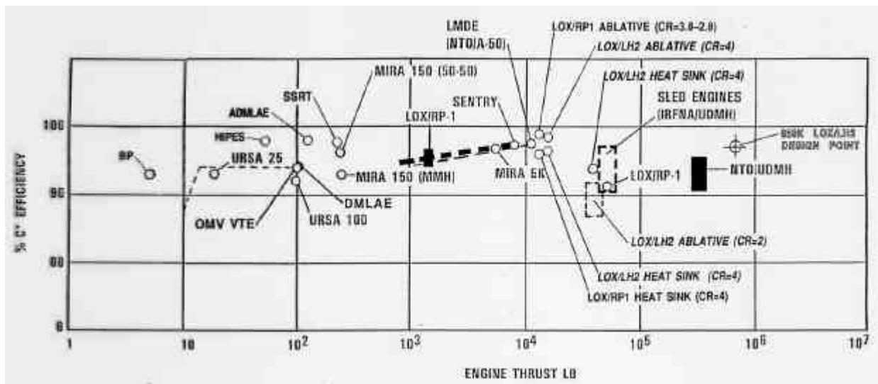
Figure 27. Summary of Combustion Efficiencies Measured on Major Pintle Engine Programs
