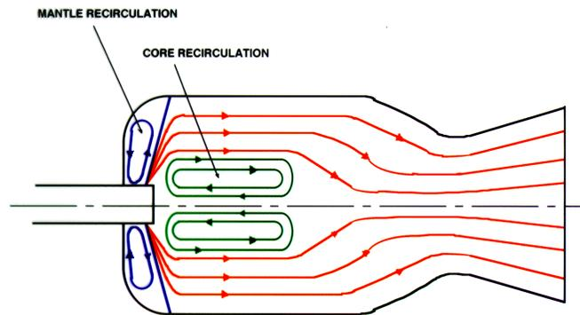
**Figure 4. Combustion Chamber Flowfield Resulting from Pintle Injection of Propellants**
