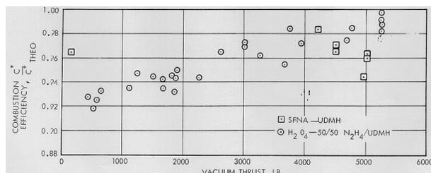
**Figure 12. Early Demonstration of Deep Throttle Capability of Pintle Injector**
