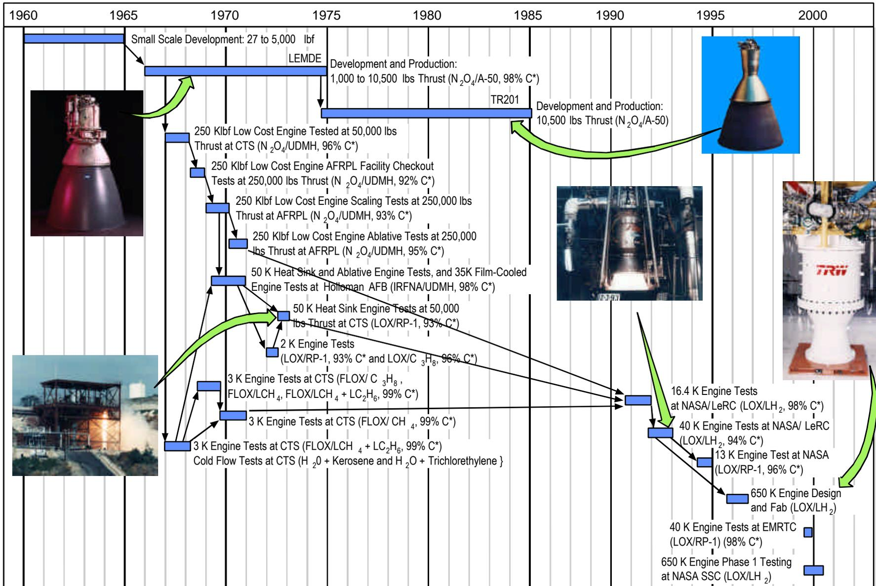
Figure 7. Chronology of Development and Production of Large Thrust (= 2000 lbf) Pintle Rocket Engine Technology at TRW
