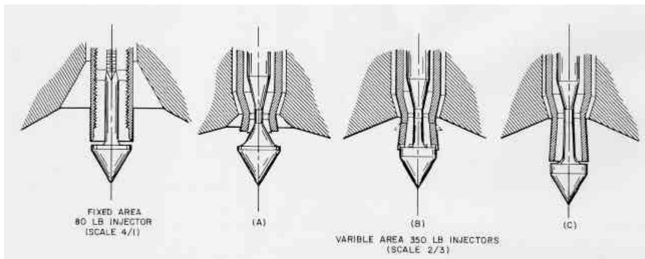
**Figure 6. Early Designs of Pintle Injector Configurations Evaluated at Space Technology Laboratories, Inc. (now TRW, Inc.), extracted from Ref. 2.**
