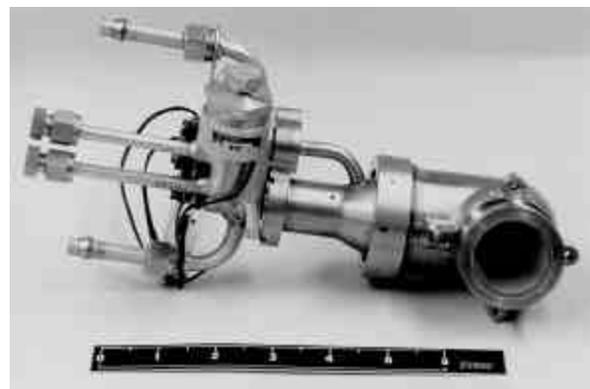
**Figure 19. KEW 10.2 Divert Thruster for Early SDI Kinetic Kill Vehicle**
