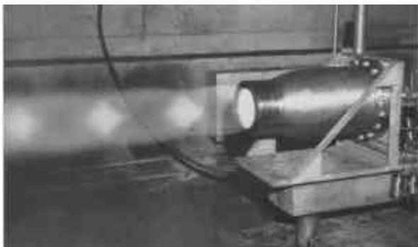
**Figure 9. Test Firing of Ablative-Cooled MIRA 5000**
