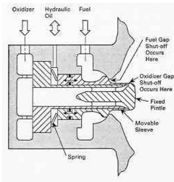
Figure 20. Face Shutoff-Only (FSO) Pintle Injector Concept Used on GESP
