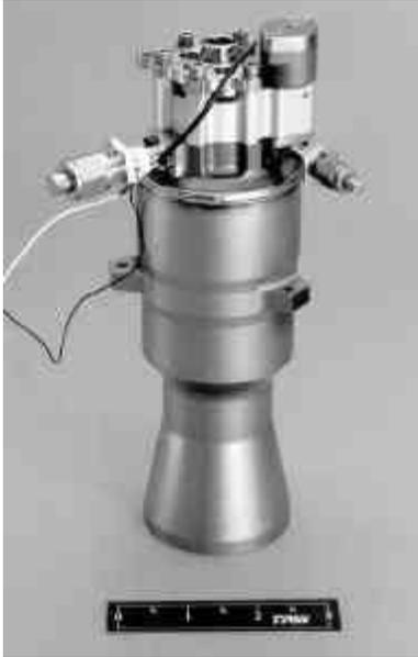
**Figure 25. FMTI Flight Engine (uses FSO pintle injector to control gel propellants)**
